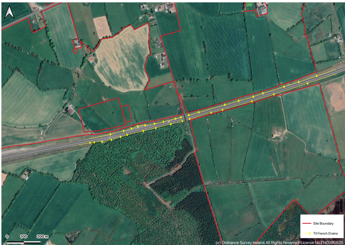
Figure 10 – French drains and their flow direction along the M6 towards Kil1
