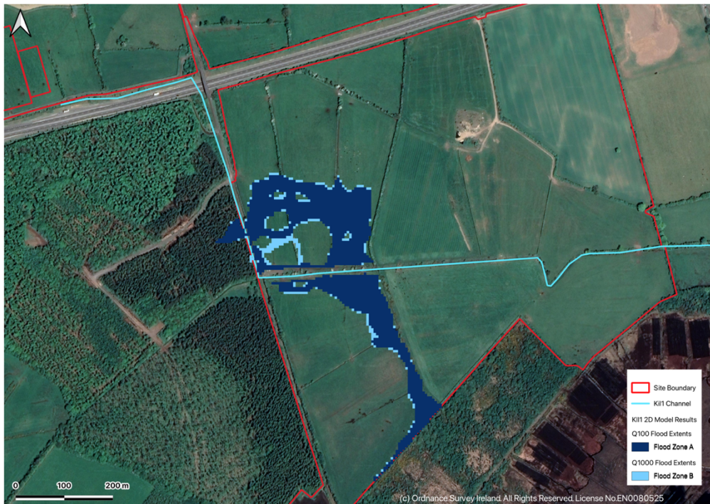
Figure 13 – Flood Extents emanating from Kil1
