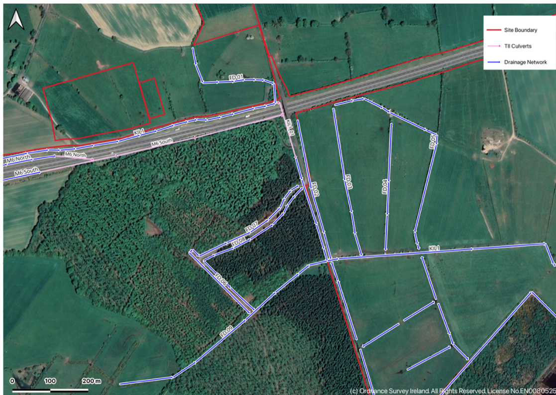
Figure 9 – Kil1 detailed drainage network
