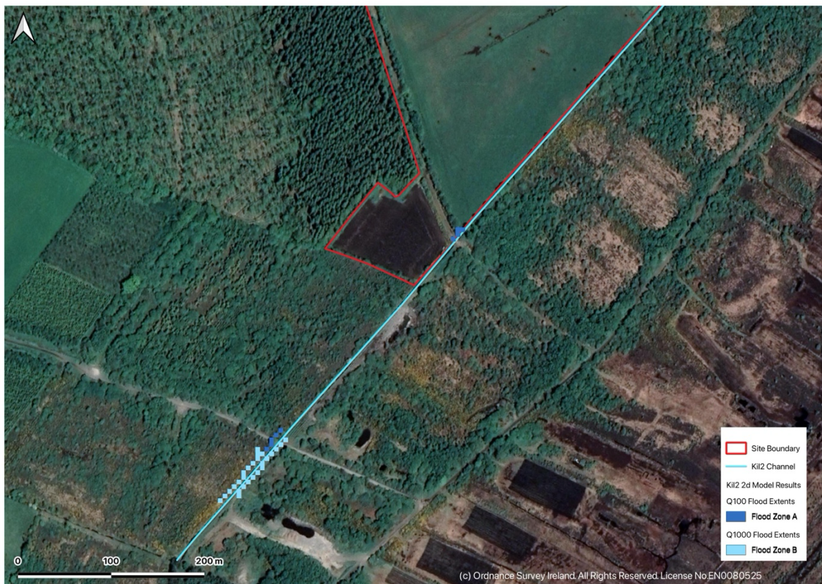
Figure 14 – Surcharging and Flood Zones adjacent to Kil2 Channel
